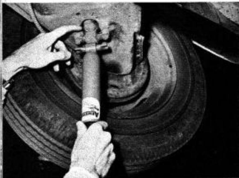
1961-1962 shock mounts sometimes require alteration to use heavier units. Opening may be enlarged by file or torch.
