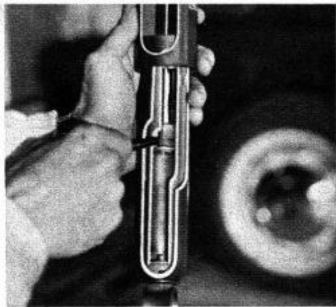
Construction of Armstrong heavy duty shock absorber is such that fluid is cooled as it is circulated and retains viscosity.
