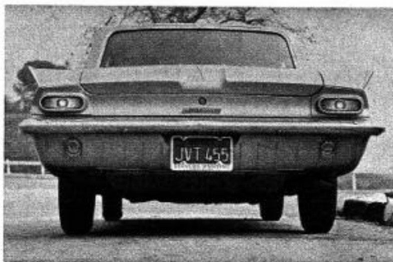
De-cambered Pontiac exhibits best road performance. Rear shows negative camber easily induced (wheels slant in at top).
