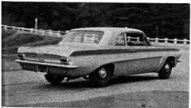
De-cambered car handled best of all Tempests tested, seems to be optimum arrangement. Right: New finned brake drums, standard on 1963 V8s offer much-needed improved braking.
